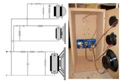
**Passive Cross-overs** Passive Crossovers are essentially a Capacitor and Coil combination, placed inside the cabinet, which filters out unwanted audio from each Loudspeaker.
