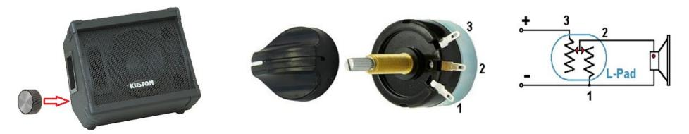
At times we find ourselves in the situation where one loudspeaker cabinet needs to be a bit louder or softer than another, but they are both on the same line. There is a simple inexpensive component called an "L-Pad" that you can get fitted to any "Passive" (no Amplifier inside) Floor Monitor. This gives you independent volume control for that cabinet.
